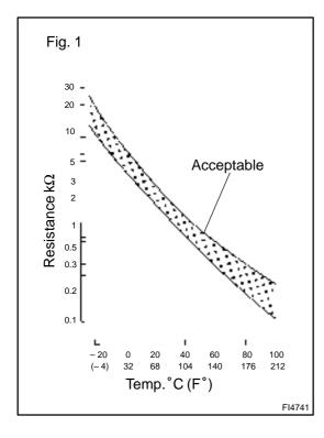
The intake air temperature sensor is built into the mass air flow meter (see page DI–23) and senses the intake air temperature. A thermistor built in the sensor changes the resistance value according to the intake air temperature, the lower the intake air temperature, the greater the thermistor resistance value, and the higher the intake air temperature, the lower the thermistor resistance value (See Fig. 1).
